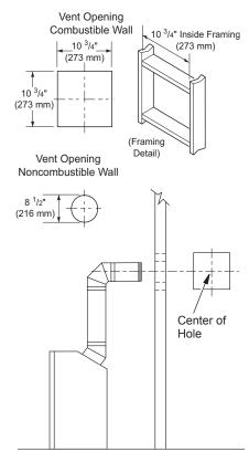
Figure 9 - Vent Opening Requirements
